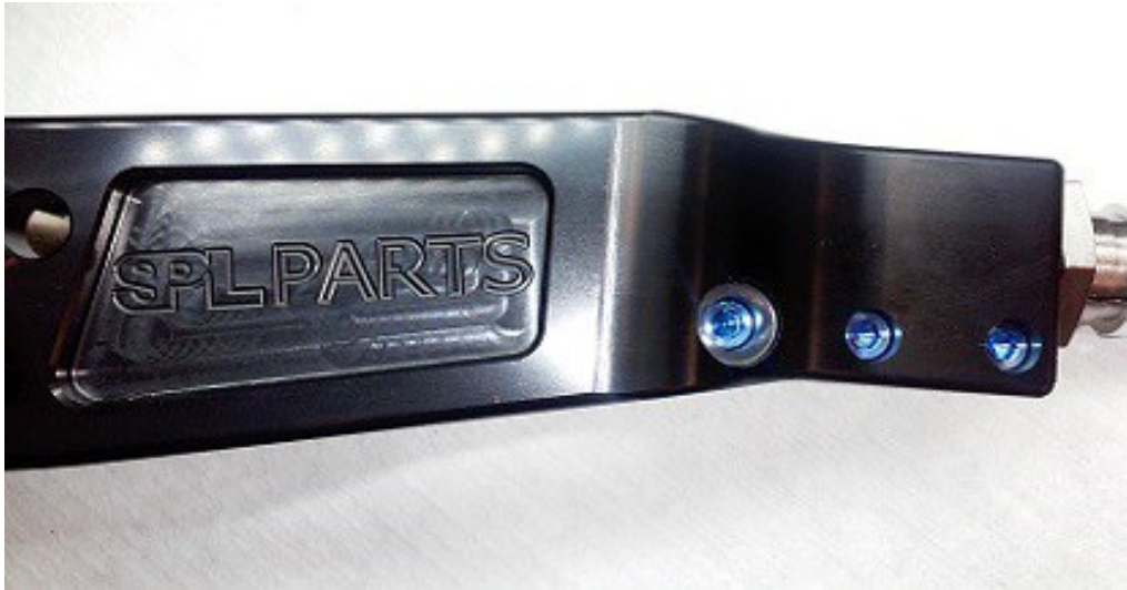
Tighten allen bolts starting from the "SPL" logo, working towards the rod end.
