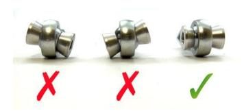
Make sure to keep the FK Rod End bearing centered during and after an alignment. The far-right image with the green check mark is the correct position.
