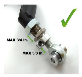
The next picture shows a properly threaded adjuster. The rod end (heim joint) will thread out about 2/3 the length of the adjuster. The maximum adjustment limits are shown in the picture. This jam nut should be tightened against the body of the arm. To properly tighten the jam nut, hold the adjuster hex with a wrench, then use a second wrench to tighten the jam nut.
