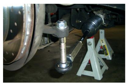
Use 2 supplied silver colored nuts, jam 2 nuts together to help hold the shank. **Torque nut on top of knuckle to 40 ft-lbs. DO NOT USE IMPACT GUN OR OVERTORQUE** otherwise strength of tie rod end will be severely compromised.
