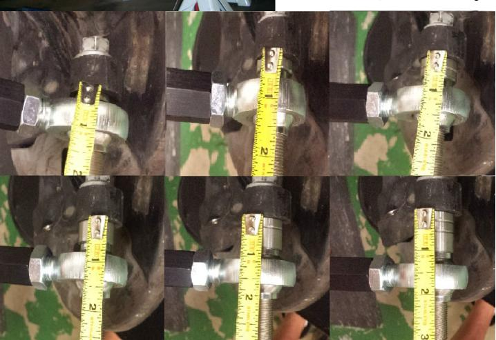
setting (2 adjustment spacer, no misalignment spacer).
