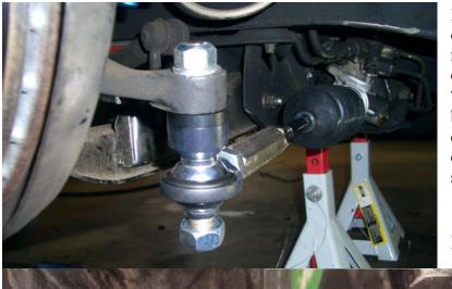
Install spacers. As pictured on left, the tie rod ends are installed with 1 adjustment spacer (flat ring spacer) and 1 misalignment spacer (large cone shaped spacer).
