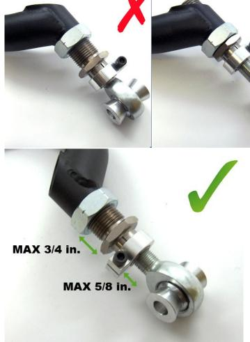
This picture shows a properly threaded adjuster. The rod end (heim joint) will thread out about 2/3 the length of the adjuster. Note also the maximum adjustment limits shown in the picture.
