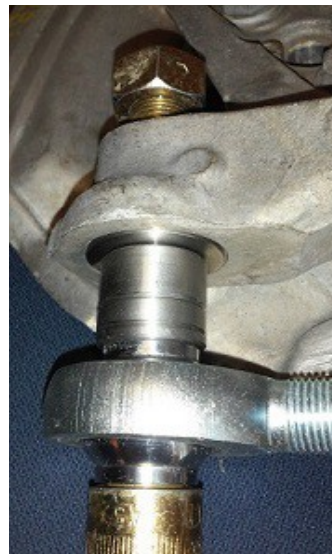
When tight, the conical spacer should be flush.
