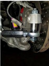
The following pictures show possible bump steer adjustment settings, using various combinations of spacers. The stock tie rod end corresponds to the setting in image #3 (with two adjustment spacers and no misalignment spacer).
