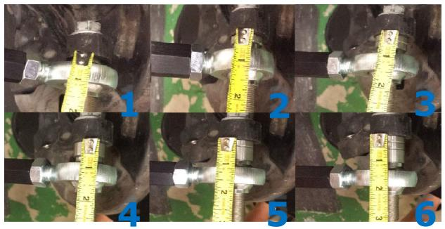
For most installations on stock knuckles, we recommend using the setting in the fourth image above (one misalignment spacer, no adjustment spacers).
