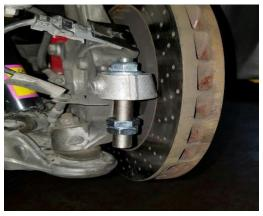
5. Remove the two nuts and install the spacers. As pictured on the left, the tie rod ends are installed with one adjustment spacer (flat ring spacer) and one misalignment spacer (large cone shaped spacer). Install the locking nut on the bottom. This nut will take some effort to thread (about 20 **ft.-lbs.** of torque) as it is a metal crimping locking nut. Torque to 80 **ft.-lbs**.
