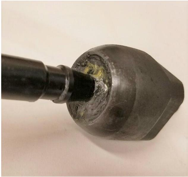
Figure 1: Factory packed grease in tie rod.
