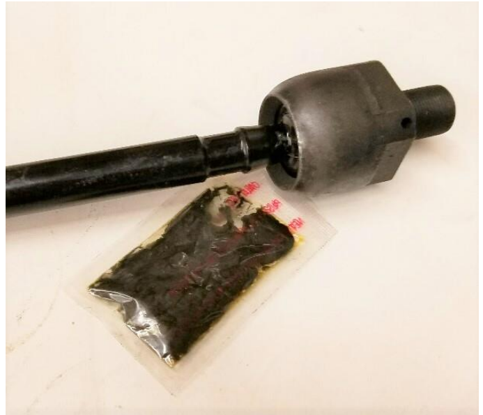
Figure 2: Factory supplied tie rod grease packets.
