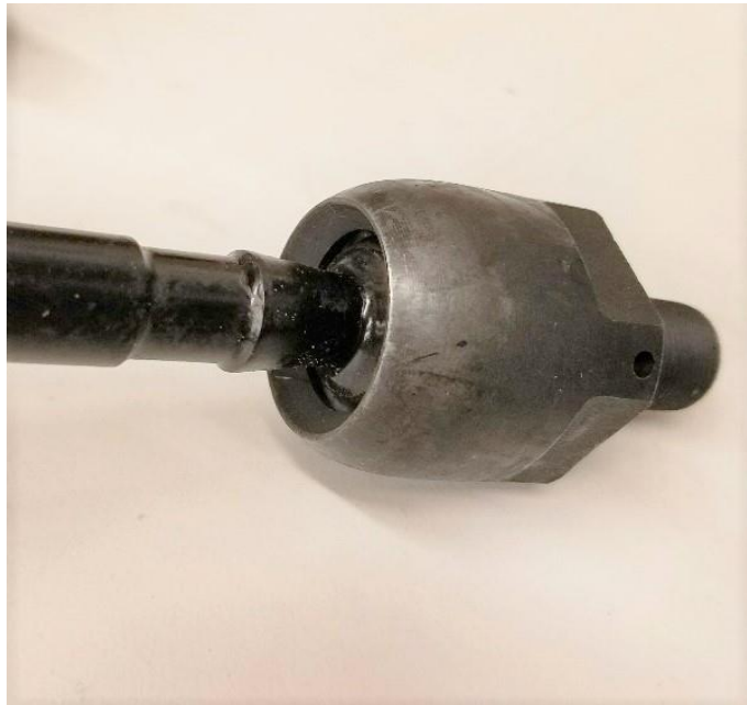
Figure 3: Dry tie rod before grease being packed into it.
