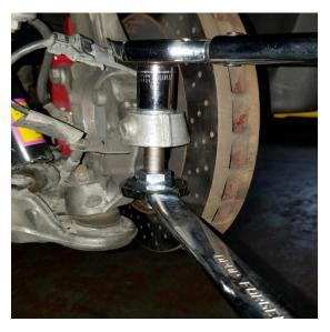
Remove the two 5/8''-18 Jam Nuts, and install the Spacers (3, 4, 5). Install the locking nut on bottom (9). Torque to 80 **ft-lbs**.
