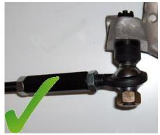
Note that the Inner Tie Rod End can rotate freely, so the picture on left is not binding even though the edge of the ball is touching the housing. If uncertain, try rotating the Inner Tie Rod by using a wrench on the hex part of the inner tie rod: Tighten down the socket head cap screws on each end of the turnbuckle until the assembly cannot rotate, not exceeding 10 ft-lb.
