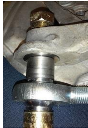
When tight, the conical spacer should be flush.
