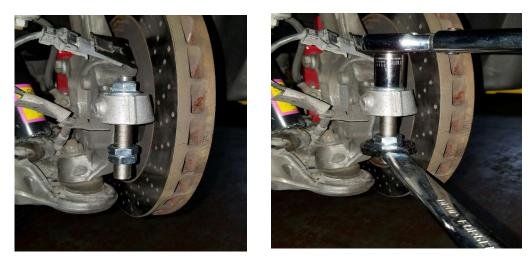
Remove the two silver colored nuts. Install supplied stainless steel spacers to adjust bump steer. You will want to try to make the angle of the tie rod set up match the angle of the lower control arm. The lower the car, the more spacers you will use. (See pictures for various combinations.) Test and adjust from there. Install locking nut on bottom. This nut will take some effort to thread (about 20 ft-lbs of torque) as it is a metal crimping/locking nut. **TORQUE TO 80 ft-lbs**.
