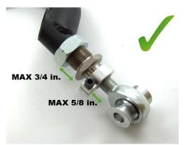
This picture shows a properly threaded adjuster. The rod end (heim joint) will thread out about 2/3 the length of the adjuster. Note also the maximum adjustment limits shown in the picture.
