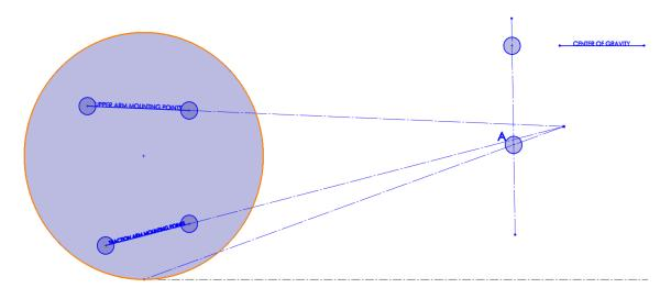
The following diagram shows what happens when you raise the subframe closer to the chassis. For this example, we are comparing what happens to the anti-squat when the ride height remains the same. When the subframe is raised, the rear "instant center" is raised as well, that moves point A up and increases anti-squat.
