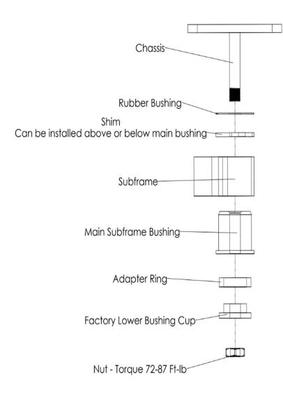
Remove subframe and OEM subframe bushings. The OEM subframe bushings can either be pressed out or cut out. The entire OEM bushing must be removed, including all the outer metal "shells" (race). When the OEM bushing is completely removed, there should just be 1 ring of steel left that is part of the subframe itself.
