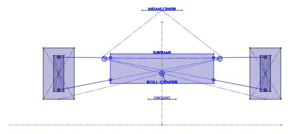
If we are to compare the 2 subframe positions with the car at the same ride height in both cases, raising the subframe will raise the roll center. **Note:** Raising the subframe will not significantly change ride height, this is because the ride height is determined by the shock/spring assembly as it sits between the chassis and the knuckle.
