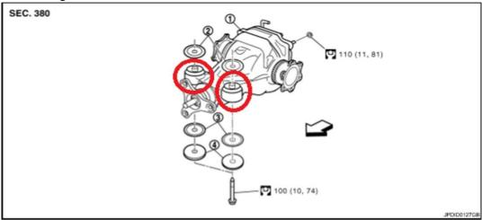
10. Remove the rear differential bushing. This one is much harder to press out, and many times must be removed with a reciprocating saw. Make sure to remove the metal ring that is pressed in around that bushing, otherwise your bearing will not press in. Be very careful when removing this to not take any material from the surface that the bearing will be pressed into.
