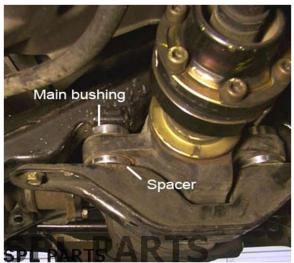
Remove the differential from the subframe and remove the OEM rear differential bushings.
