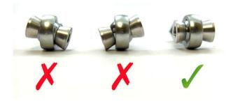
5. Once installed, ensure that both of the FK Rod Ends (4, 5) are centered and have full articulation. Lock them in place by tightening the Blue Titanium Socket Head Cap Screws (7) with a 3/16 allen wrench to 150 **IN. lbs.**
