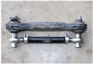
4. Install the SPL Parts Arm using the OEM hardware. Please ensure the Tapered Stainless Steel Spacer (2) provided mates up with the tapered section of the knuckle. Tighten the nuts to 73.7 **ft. lbs.** (100 N/M) at both ends. **DO NOT OVERTORQUE!** SPL Parts is not liable for any issues due to overtorque.
