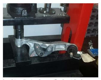
A 1 1/8-inch socket will be a useful driver to install the bushings (we happen to have a differential bushing driver on hand) pressing them in almost to the point of the lip being flush with the arm, keeping the gap from lip to arm slightly larger than the retaining clip lip gap. By doing so, you will prevent marring or crushing the retaining clip end of the bushing. Line up the bushing, making sure it is straight with the bore of the arm. Once the
