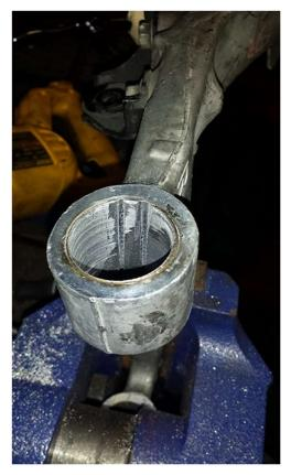
Note the two cuts in bushing sleeve
