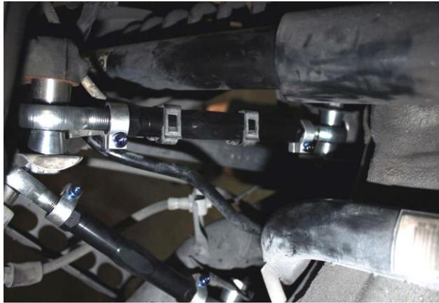
6. Attach the ABS sensor wire clips to the SPL Parts arm.
