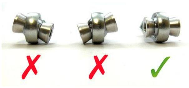
5. Once installed, ensure that both of the FK Rod Ends (2, 3) are centered and have full articulation. Lock them in place by tightening the Blue Titanium Socket Head Cap Screws (6) with a 3/16 allen wrench to 150 **IN. lbs.**
