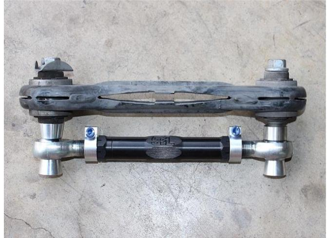
3. Install the SPL Parts Arm using the OEM hardware.. Tighten the nuts to **73.7 ft. lbs.** (100 N/M) at both ends. **DO NOT OVERTORQUE.** *SPL Parts is not liable for any issues due to overtorque.*
