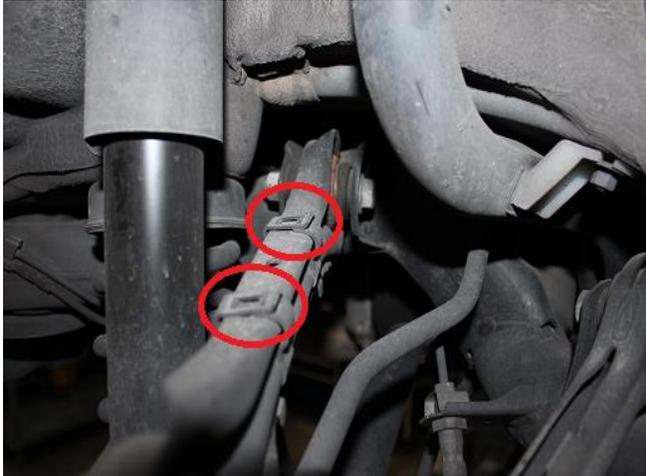
1. Using a flat head screwdriver, remove the clips attaching the ABS sensor wire from the OEM arm.
