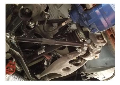
The SPL RTR F8X is designed to remove the deflection caused by rubber bushings, and allow for a wide range of easy adjustment to dial in your suspension for whatever type of driving you are doing, whether it be down winding back roads or on the track. Below are the installation instructions. Make sure to adhere to these closely, otherwise you may damage your part, reduce the life of the rod ends, or damage other components of your suspension.
