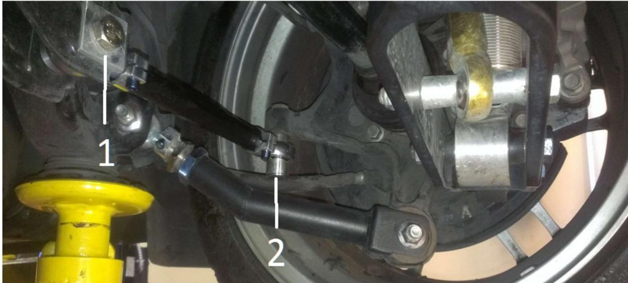
1. If you are reusing the OEM eccentric nut and bolt, mark the location with a marker allowing you the reinstall in the exact same location.
