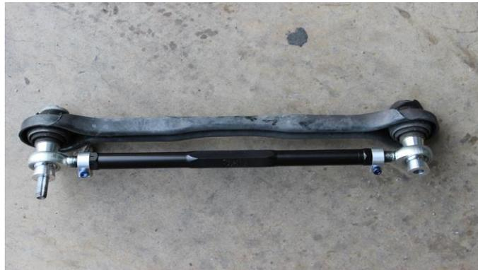
2. Set SPL Parts Rear Toe Arm next to the OEM arm. Use the bolts through the stock arm to set the SPL Parts Arm to the exact length of the OEM arm ensuring equal thread engagement on both ends. **Note:** the groove on one side of the arm to indicate the left-hand threaded side.
