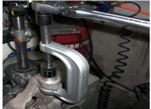
Press out stock bushing using appropriate bushing press and driver.
