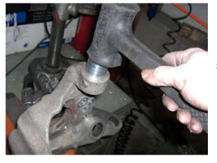
Lightly tap new bushing in place to start, making sure bushing is square against the bore.
