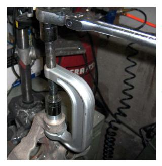
Press in new bushing completely with appropriate press and driver.
