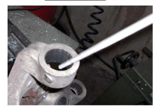
If the side of the knuckle which the new bushing goes in is not chamfered, use a round file to break the edge.
