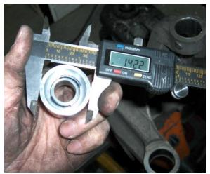
4. Measure the diameter of the new SPL Parts bushing. Confirm that the new bushing is between 1/1000 and 3/1000 inch (0.025mm to 0.076mm) larger than the bore on the knuckle. If this tolerance is out of spec, please contact us for a replacement bushing.
