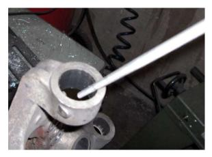
5. If the side of the knuckle which the new bushing goes in is not chamfered, use a round file to break the edge.
