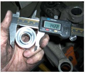
4. Measure the diameter of the new SPL Parts bushing. Confirm that the new bushing is between 1/1000 and 3/1000 inch (0.025mm to 0.076mm) larger than the bore on the knuckle. If this tolerance is out of spec, please contact us for a replacement bushing.
