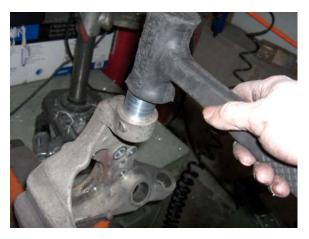
6. Lightly tap the new SPL Parts bushing in place to start, making sure the bushing is square against the bore.
