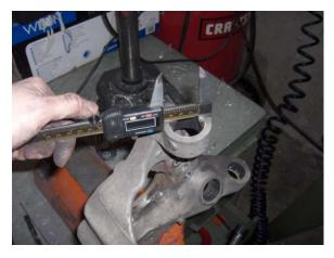
3. Measure the bushing bore of the knuckle.
