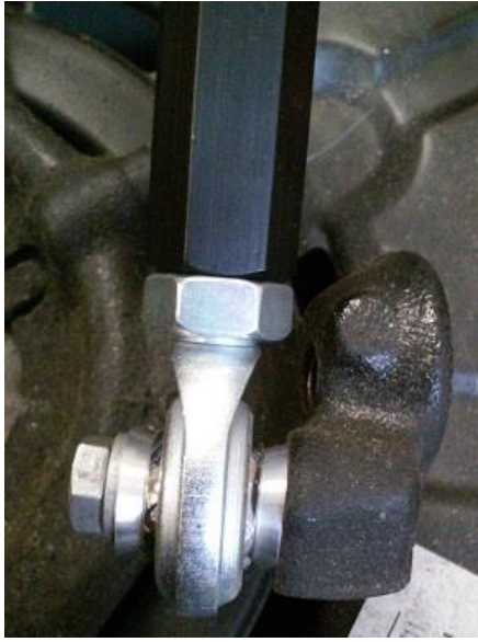
Proper installation of spacers at knuckle.
