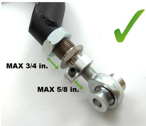
This picture shows a properly threaded adjuster. The rod end (heim joint) will thread out about 2/3 the length of the adjuster. Note also the maximum adjustment limits shown in the picture.
