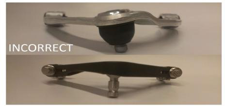
The images above show the correct way to determine what arm goes on what side of the vehicle. Match up the SPL arm with the OEM arm by observing the canted ball joint. This will allow proper articulation of the ball joint.
