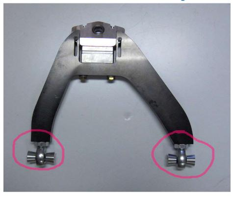
Caster adjustment must be pre-set before installing the arms to the car. It is not adjustable on the car, so the arm has to be disconnected to set caster.
