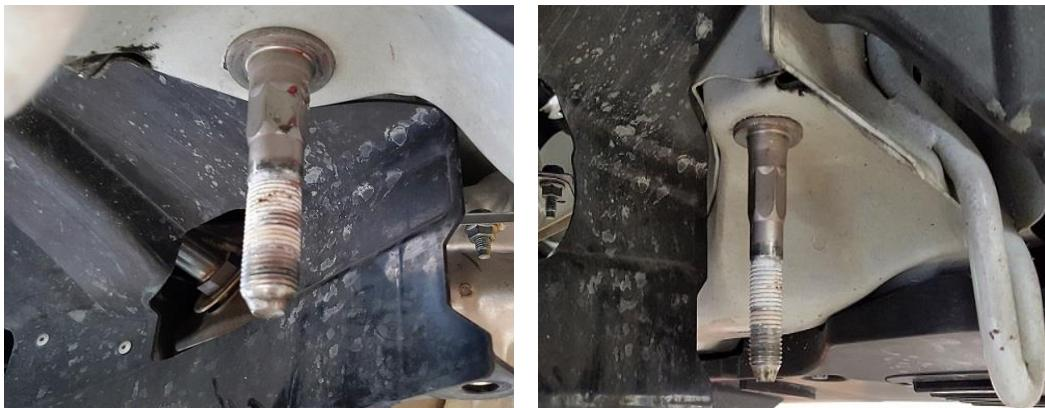
6. Install the SPL Parts Control Arm at subframe end first. The large Offset Spacer should go to the rear of the car, and the small offset spacer to the front of the car on the joint. Place the bolts through, but do not tighten yet as this will make it more difficult to finish the installation.
