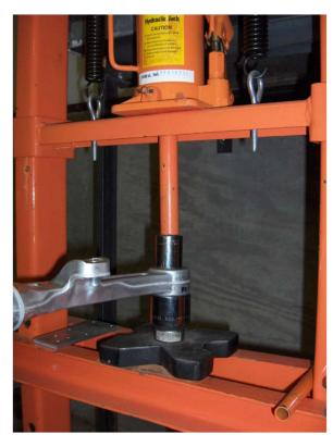
1. Press out stock bushing using appropriate bushing press and driver. For reference, the following Sears/Craftsman sockets will work as the driver and receiving cup:
