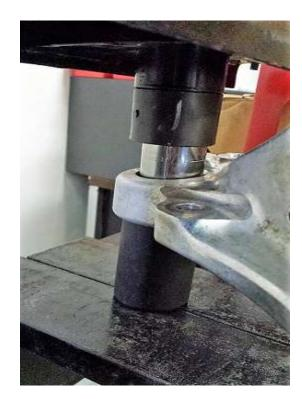
Press out stock bushing using appropriate bushing press and driver. As shown, we used a 1 1/8 inch socket as the driver. Also keep the flat side of the arm facing down.
