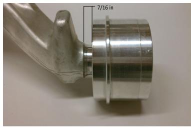
4. Press the bracket onto the new SPL Parts bushing. Be sure to press it in with the same orientation as the stock bushing so it will mount properly to the chassis. You may need to press the bushing onto the arm a bit more to get the bolt holes for the bracket to line up.
