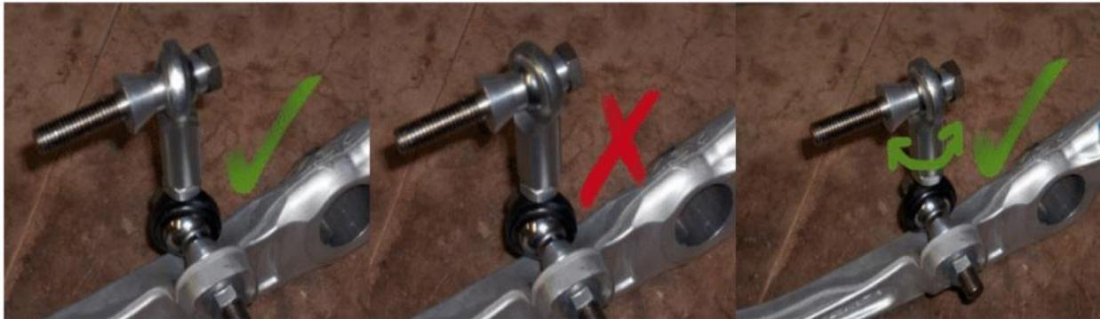
7. Once both sides of the sway bar are attached without any preload induced into the system, tighten down both sides to 30 **ft.-lbs.**
