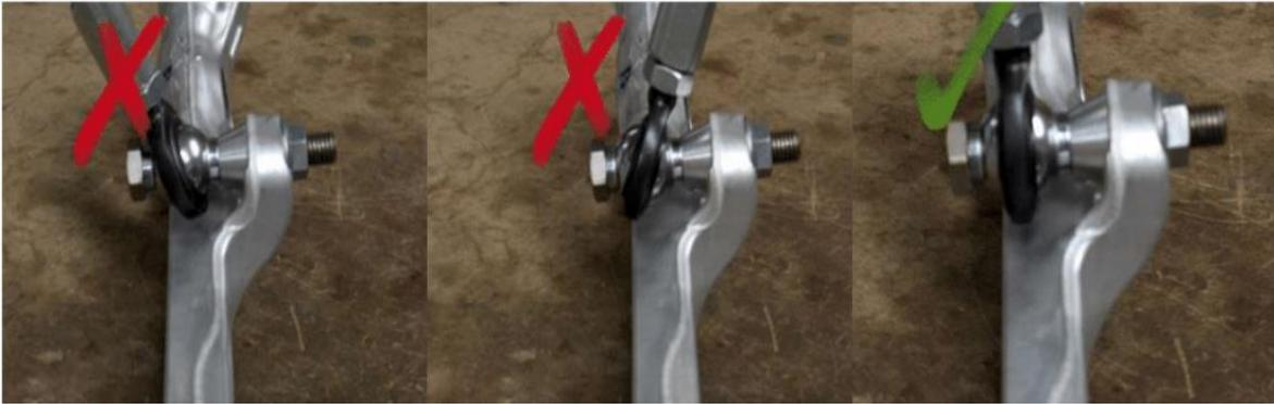
5. Install the end link on the other side of the vehicle onto the sway bar. Adjust the length of this end link so you do not have to apply any force to the sway bar or control arm to install the stud. As shown in the images below, the stud should line up well and slide through easily. If you are unable to achieve this, change the length of the end link on the other side of the vehicle and try again.
