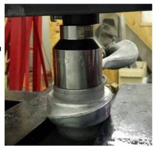
or burrs. The same socket can then be used to drive in the new bushing. Again, make sure to align the driver and bushing to go in straight and not bind.
