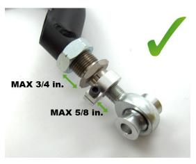
This picture shows a properly threaded adjuster. The rod end (heim joint) will thread out about 2/3 the length of the adjuster. Note also the maximum adjustment limits shown in the picture.
