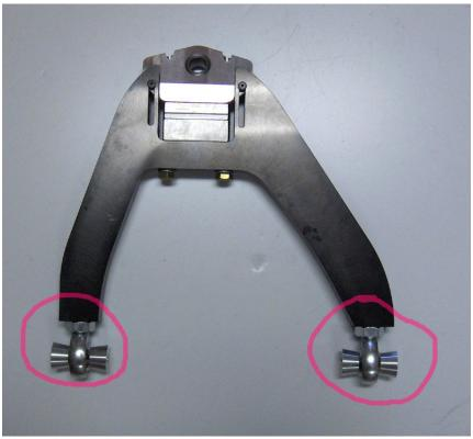
Tighten nut (15/16" hex) connecting arm to spindle to 40 ft-lbs.
