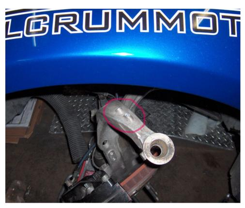
Remove stock front upper arms. **IMPORTANT** Locate the 2 casting "bumps" on the back of the upright (shown circled in picture). Grind off the bumps till smooth. This is important in order for the arms to have maximum suspension travel.
