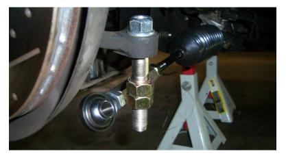
Use 2 supplied silver colored nuts, jam 2 nuts together to help hold the shank. **Torque nut on top of knuckle to 40 ft-lbs. DO NOT USE IMPACT GUN OR OVERTORQUE** otherwise strength of tie rod end will be severely compromised.
