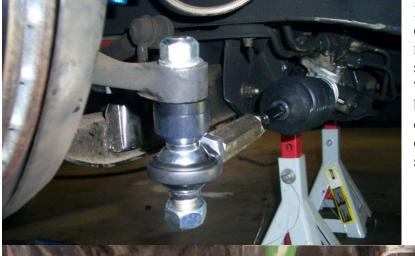
Install spacers. As pictured on left, the tie rod ends are installed with 1 adjustment spacer (flat ring spacer) and 1 misalignment spacer (large spacer).
