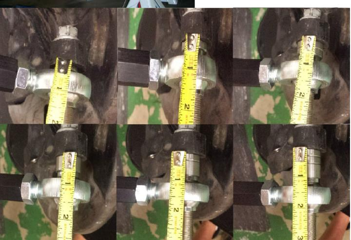
For most installations on stock knuckles, we recommend using 4th setting (1 misalignment spacer, no adjustment spacers).
