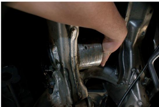
Method 2: Using an appropriate “receiving cup” and clamp, press the OEM bushing out with the subframe on the car. As in method 1, orient the smaller diameter end of the driver tool towards the subframe bushing to self-center the driver on the OEM bushing race.
