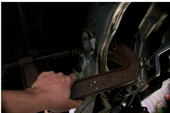
**DO NOT TORCH THE OEM BUSHING!** Applying heat can alter the temper characteristics of the aluminum subframe and significantly weaken it. This applies to 350Z only, all 370Z including Nismo editions have steel subframes.
