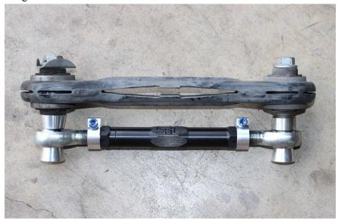
4. Install the SPL arm using the OEM hardware. Please ensure the tapered Stainless Steel spacer provided mates up with the tapered section of the knuckle. Tighten the nuts to 73.7 Ft Lbs (100 N/M) at both ends.
