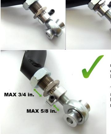
This picture shows a properly threaded adjuster. The rod end (heim joint) will thread out about 2/3 the length of the adjuster. Note also the maximum adjustment limits shown in the picture.
