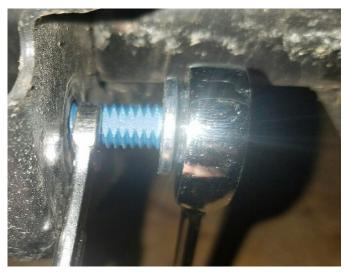
3. Insert Rod end and spacers between inner chassis mounts and insert threaded rod from the back of the car towards the front with the flat towards the back of the car. With a crescent wrench or 5/16 wrench, hold the flat of the threaded rod and tighten the locknut with the 15mm wrench/gearwrench/socket.
