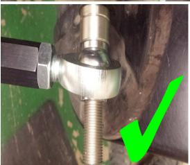
Note that the toe arm rod end can rotate freely, so the picture on left is not binding even though the edge of the ball is touching the housing.
