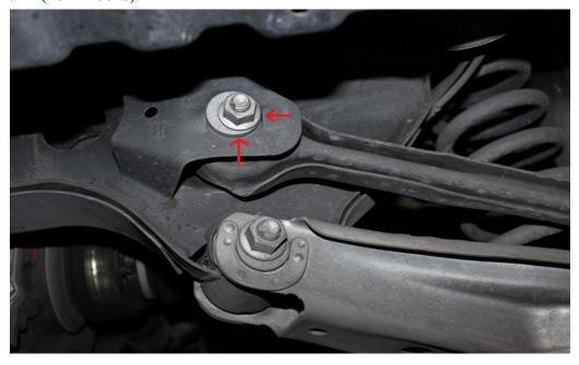
2. Set SPL arm next to the OEM arm. Use bolts through the stock arm to set the SPL arm to the exact length of the OEM arm ensuring equal thread engagement on both ends (picture 2). Note the groove on one side of the arm to indicate the left hand threaded side.
