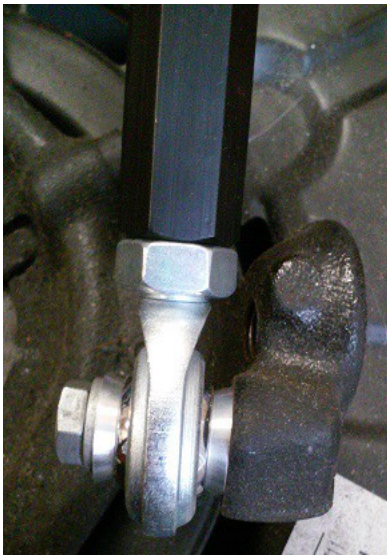
Illustration 2: Proper installation of spacers at truckle
