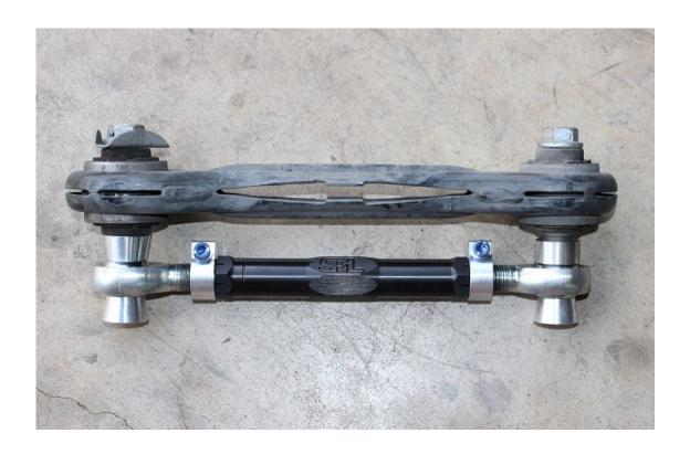
3. Install the SPL arm using the OEM hardware. Please ensure the tapered spacer provided mates up with the tapered section of the knuckle. Tighten the nuts to 73.7 Ft Lbs (100 N/M) at both ends.
