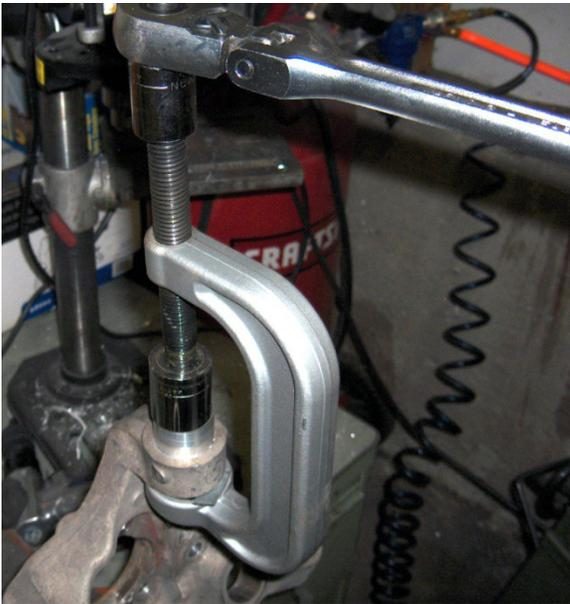
Press in new bushing completely with appropriate press and driver.
