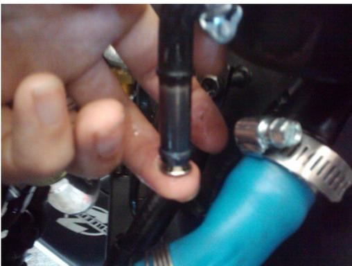
Install metal plug onto barb for return hose of Hicas system on the power steering reservoir.
