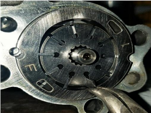
Remove pump vanes by using needle nose pliers to remove them.
