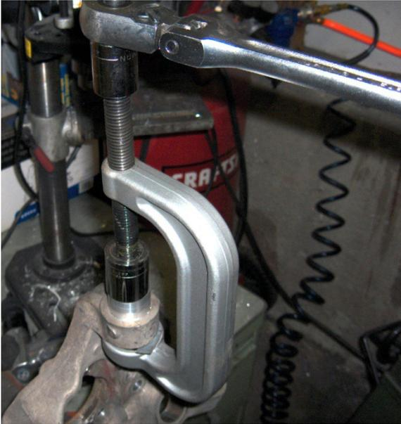
Unbolt rear retaining washer on the Hicas ball joint. Press out stock Hicas ball joint using appropriate bushing press and driver.
