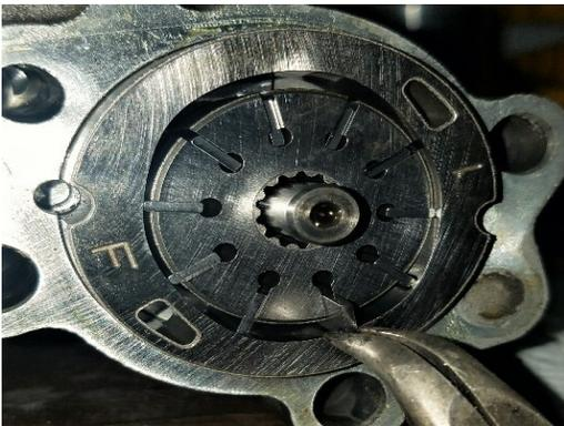
Remove pump vanes by using needle nose pliers to remove them. Reinstall back cover, torque to 23-31 ft-lbs.
