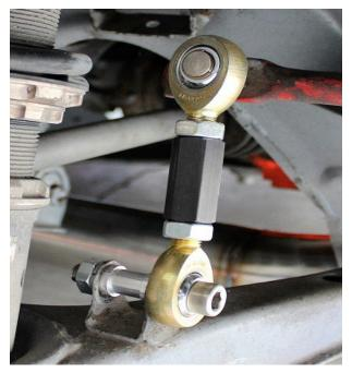
It is important to ensure that the endlink has good articulation, because as the suspension moves up and down the sway bar endlink needs to move in an arc. First check that the lower spherical bearing still has sufficient articulation. The following pictures demonstrate bad installation angle (first 2 pics) vs. good installation:
