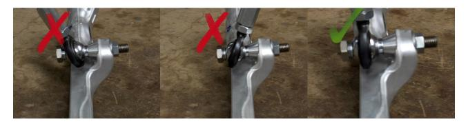
It is also important to ensure the endlinks have good articulation in another direction of motion – the twisting motion, as seen below:
